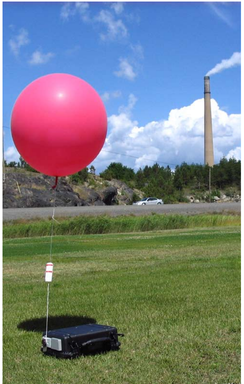
Bestech's remote control weather balloon launcher in forefront of Vale Inco Superstack in Sudbury.
